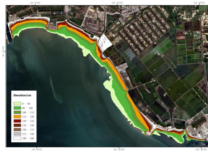
Figure 4. Approximate topography build of tidal flat using tide level contour and TIN in test area.
